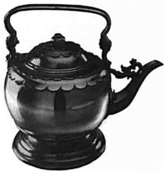
PLATE 27b White-brass kettle casted in Terengganu using the lost-wax process. (Photo: courtesy of Malaysian Handicraft Development Corporation)
